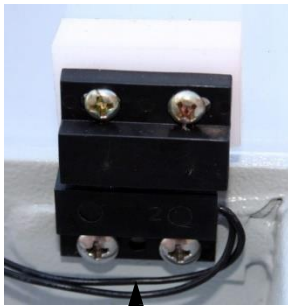
Safety cut-off switch
