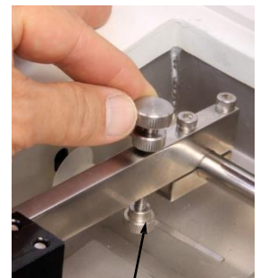
Adjust mechanical cut-off height every time the flange size is changed
